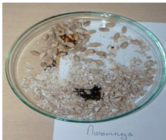
Sl.2. Reakcija povidin-joda u kontaktu sa usitnjenom pšenicom i onom koja nije usitnjena Fig.2. Reaction of povidin-jode in contact with ground wheat and one that is not chopped
