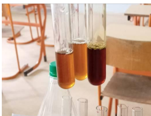
Sl.1 Promena boje zelenog čaja po dodatku kiseline i baze Fig.1 Change of color of green tea after the addition of acid and base
