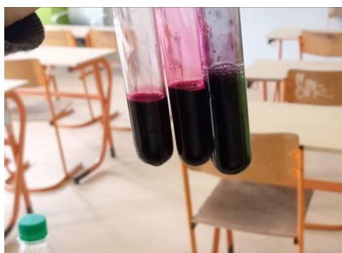
Sl.1 Promena boje hibiskusa po dodatku kiseline i baze Fig.1 Change of hibiscus color after the addition of acid and base
