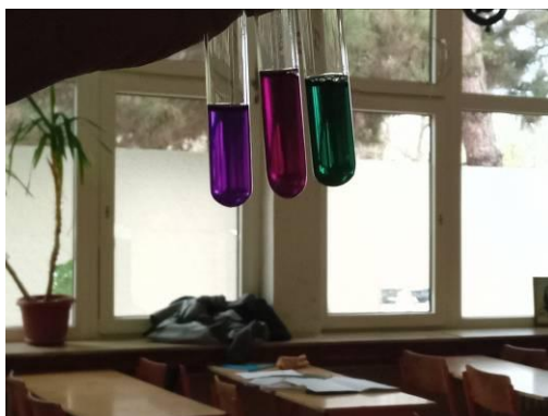
Sl 1 Promena boje crvenog kupusa po dodatku kiseline i baze Fig. 1 Color change of red cabbage after the addition of acid and base
